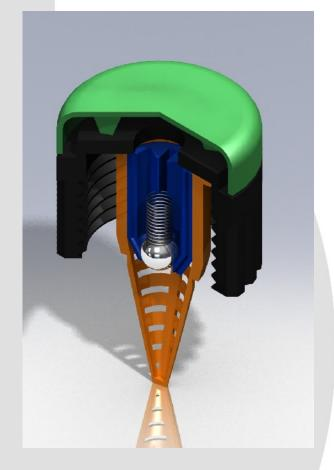
The per-perimetry utilizes spring check valve technology to create a true check valve with a 4 PSI cracking pressure. This saves water by eliminating low head drainage for up to a 9.25 foot elevation change. The combination of the Spec-Check along with GPH's GPST & GPCB ensures that your system will operate at the highest level of performance and efficiency.
